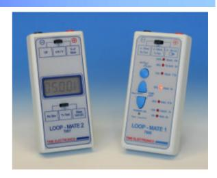
The Loop-Mates are single function low-cost pocket sized units, designed for test and calibration of process loops. Simplicity of operation is their key - no keypads or complicated selections. Engineers will be able to pick them up and get to work immediately. Just select 4 - 20mA, or 10V loop, and TxSim, RxTest, RxSim or TxTest. Both have internal loop drive supplies which can be used to power the loop if required.
